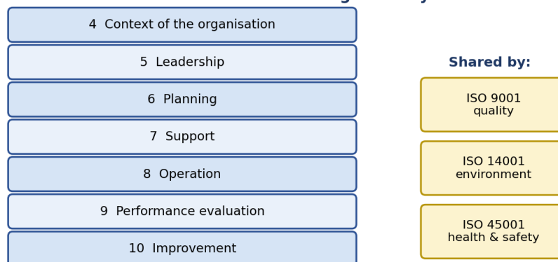
Figure 2.9 — The common structure of management system standards (Annex SL)
